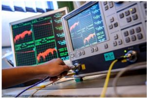
Note that for specific multi-antenna and multi-channel applications, the phasing between coax cables assemblies, also called "phase matching", is a key step in the proper functioning of the system. The phasing of the signals implies an identical electrical length for each coax cable assemblies and therefore a very precise cutting capacity. In practice, this requires a resumption of the length of each cable after an intermediate RF measurement.
